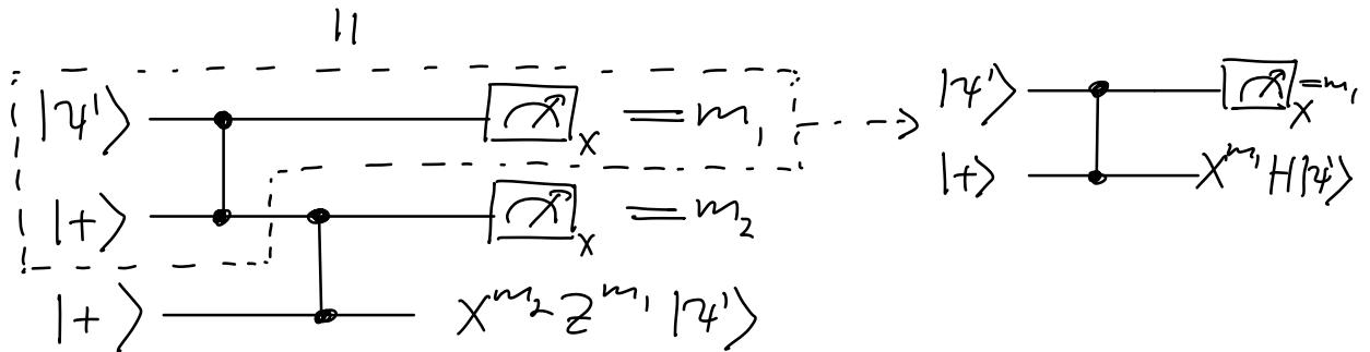
A single-qubit  $Z$  rotation  $e^{i\theta Z}$  can be implemented in a teleportation-based way:
